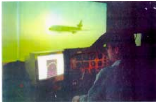
Figure 1. The simulation environment, showing the CDTI to the left and the instrument panel (IP) to the right.
